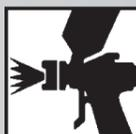
Set up/Air pressure 1.3-1.4mm 1.5-1.8 Bar
