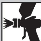
Set up/Air pressure 1.3-1.4mm 1.5-1.8 Bar
