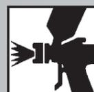
Set up/Air pressure 1.3-1.4mm 2-2.3 Bar
