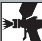
Set up/Air pressure 1.3-1.4mm 2 Bar
