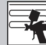
Apply medium to wet closed coat, flash, followed by a full coat
