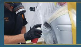
Apply 3-4 coats of the topcoat colour. Apply light even coats to build up the colour to achieve full coverage. Allow 2-3 minutes between each coat. Extend the application of the topcoat an additional 10-15cm into P1000 the sanded area. Allow to dry for 30 minutes.
