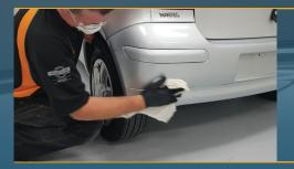
First wash your car to remove all dirt and grime from the repair area. Allow to dry. Clean all surfaces to be painted using clean rags and a quality wax and grease remover (such as Valspar Refinish 155 Surface Cleaner). Use a two rag method to wipe on and wipe off to remove all contamination including grease, oil, silicones, waxes etc.
