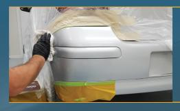
Once the surface is completely dry, remove the masking film to reveal the repaired paint area. Inspect the repair area for any dust or dry spray. If contamination is present, lightly sand out defects using P1000-P2000 and clean water.
