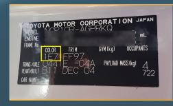
Identify the topcoat colour required by retrieving the paint code from the compliance plate typically located in the engine bay or door jam. Ensure you know the car code, make, model and year. The paint shop staff will fill an aerosol with the topcoat colour specific to your vehicle. NOTE: This process is designed for most solid or metallic colours. Special effect colours will need to be repaired by a qualified repairer.
