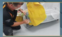
Mask around the repair area with tape and paper to protect the rest of your vehicle. Be sure to leave 10-15cm additional space for overlap with the existing coating.
