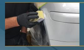
Dry sand the damaged area with P180, P240 then P320 paper.
