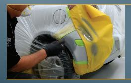
Apply 2-3 coats of Valspar Grey Shade Aerosol Primer to the damaged area. Apply light coats allowing 2-3 minutes between each coat (or until touch dry). Extend the primer application 10-15cm beyond the damage area, keeping within the sanded area. Allow the primer to dry for a minimum of 20 minutes. Note: Shake the aerosol can thoroughly for 2-3 minutes before application.
