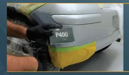
Using a small sanding block, sand the primer with P400 or P500.
